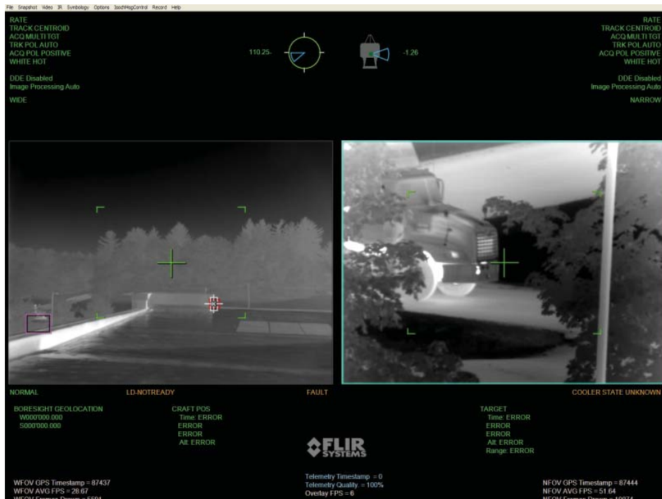
Screenshot displays Wide FOV image (left) and Narrow FOV (right). Actual WFOV and NFOV IR imagery shown on the Sensor Control Unit (SCU.)
